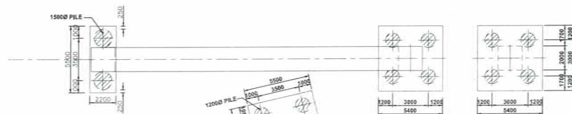
CROSS SECTION AT 10-10 (A Ramp PIER 34)
