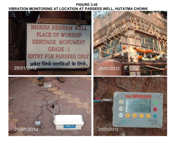
The graph has been plotted for radial, transverse and vertical vibration and shown in **Figure 3.46**, **Figure 3.47** & **Figure 3.48** respectively. The result of the monitoring shows that, the average radial vibration is about 86 VdB and the peak radial vibration is 88 VdB. The average transverse vibration is found to be 81 VdB and the peak transverse vibration is 83 VdB. The average vertical vibration is 107 VdB and the peak vertical vibration is found to be 113.9 VdB.
