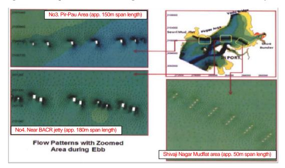
Source: The Central Water and Power Research Station (CWPRS) Technical Report No.5165 (Mar, 2014) Figure 6.2.13 Flow pattern around Piles of MTHL Bridge during Ebb Tide
