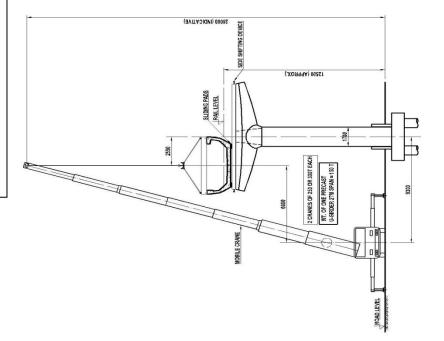
STAGE 2 - INSTALLATION OF U-BEAM ON PIER CAP SECTION B-B SALE: 1780
