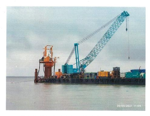
Photo No. 7: 3m dia pile boring at MP 173A LHS in progress
